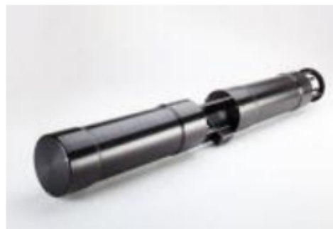
Detail of the LISST-VSF optics path, showing the receive optics and the Roving Eyeball
