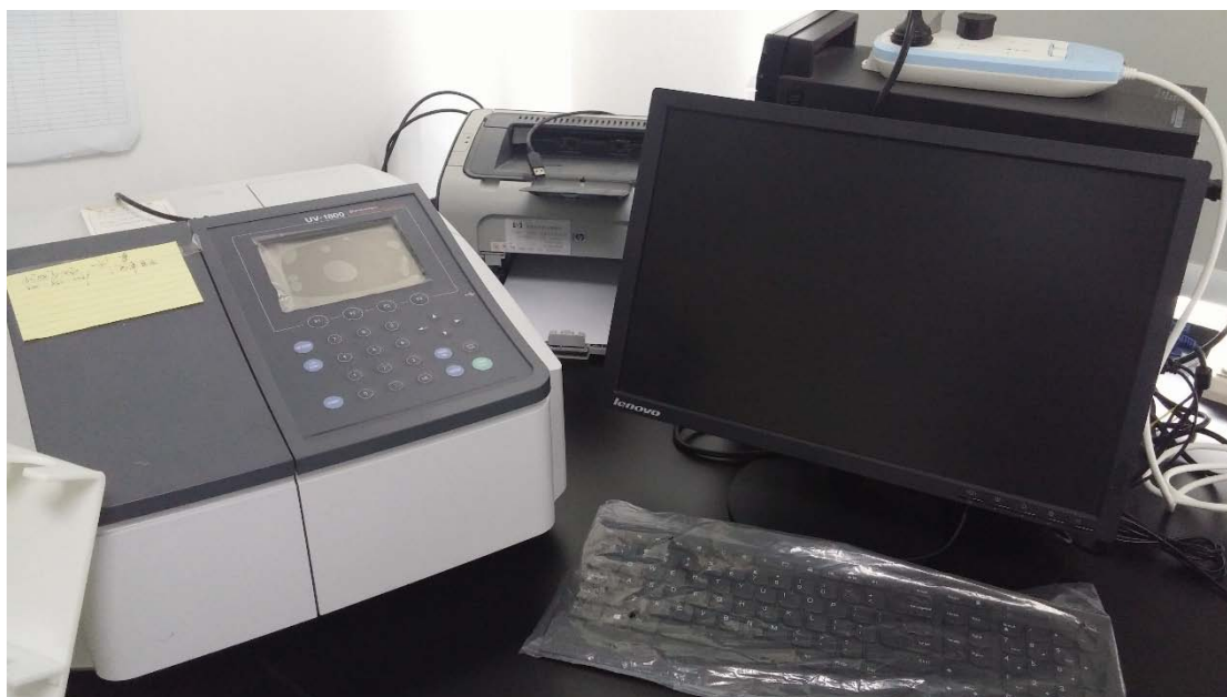
Picture 13 紫外可见分光光度计 (DU800UV/VIS)
