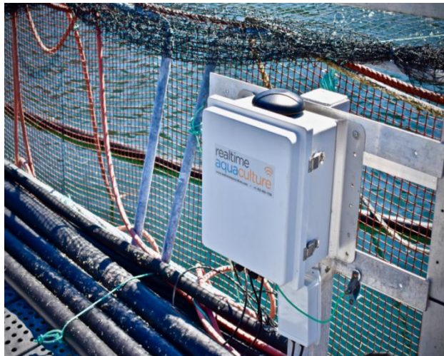
Fig. 7: HUB Wireless Sensor/Data Logger ( www.innovasea.com )
