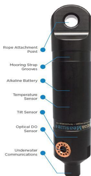
Fig. 1: Dissolved Oxygen and Temperature (DOT) Wireless Sensor/Data Logger ( www.innovasea.com )
