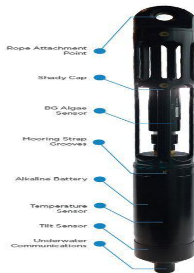
Fig. 3: BGA (Marine) Wireless Sensor/Data Logger ( www.innovasea.com )
