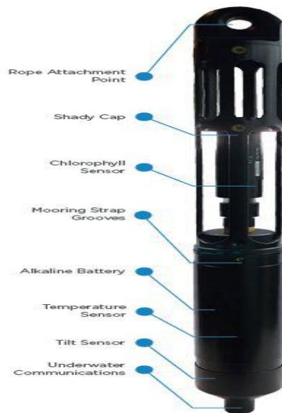
Fig. 5: CHLA Wireless Sensor/Data Logger ( www.innovasea.com )
